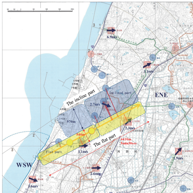
Fig.9 Estimated radiation area from thunderclouds on Apr. 8, 2018. Yellow area : The flat part of thunderclouds Blue area : The incline part of thunderclouds Wind direction and wind velocity : Average value (6:50 ~ 7:00) at 13 m above the ground
